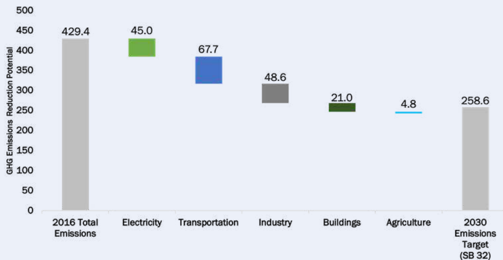
Figure S-2 Identified Emissions Reduction Potential for Meeting the 2030 Targets by Sector (MMTCO 2 e)
