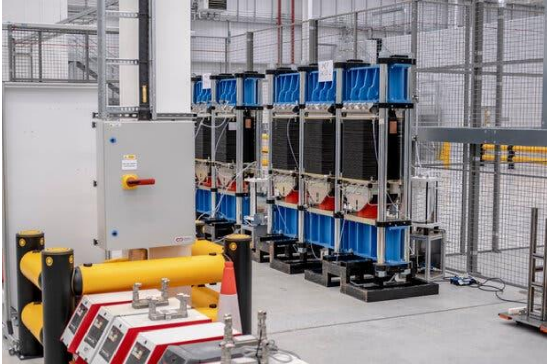
Testing electrolyzers at a green hydrogen project in Sheffield, England. Credit: Andrew Testa for The New York Times
