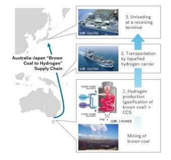
Australia is expected to be a major hydrogen supplier to Japan. The first trip was successfully completed using liquefied hydrogen. The hydrogen was produced from coal in Australia. Source: See first figure mention in text for source.
