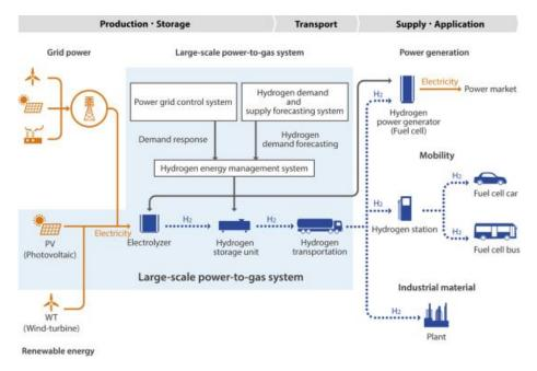
The Fukushima Hydrogen Energy Research Field (FH2R) project is testing how to use hydrogen to power stationary fuel cell batteries to provide energy storage to the power grid in a large-scale power-to-gas system. Source: See first figure mention in text for sources.
